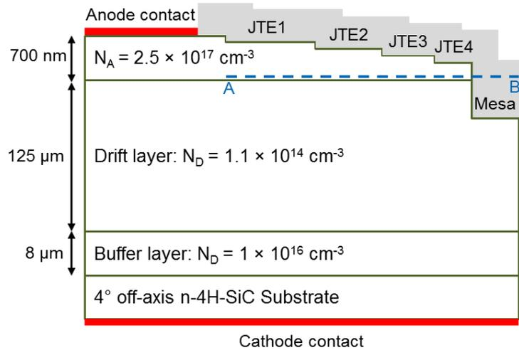
Fig. 1. Schematic cross-sectional view of the fabricated 4H-SiC PiN diodes with the O-JTE.
