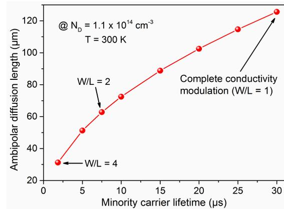
Fig. 3. Calculated ambipolar diffusion length ( $L$ ) versus minority carrier lifetime ( $\tau_p$ ).
