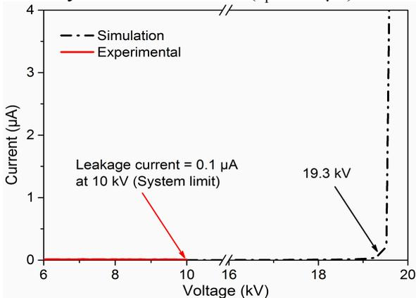
Fig. 4. Measured and simulated reverse characteristics of the fabricated PiN diodes at room temperature.
