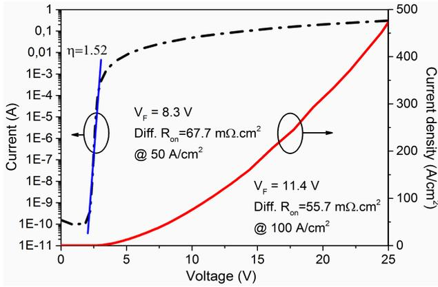
Fig. 2. Measured  $I-V$  forward characteristics of a fabricated test PiN diode, shown with logarithmic (left) and linear (right) scales.
