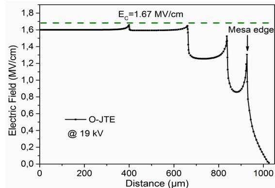
Fig. 5. Simulated electric field distribution for the O-JTE at the reverse bias of 19.3 kV. The dashed line indicates the critical electric field for SiC according to [16].
