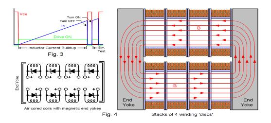
With the end yokes the inductance/disc remains constant as more discs are used, and the effective clamp diode's voltage and current capability automatically matches that of the inductor, for any arrangement of series and parallel connections. This test circuit can also be used to measure avalanche energy during the first turn-off, either by removing the clamp diodes, or with clamp voltage set above the transistor's avalanche level.
