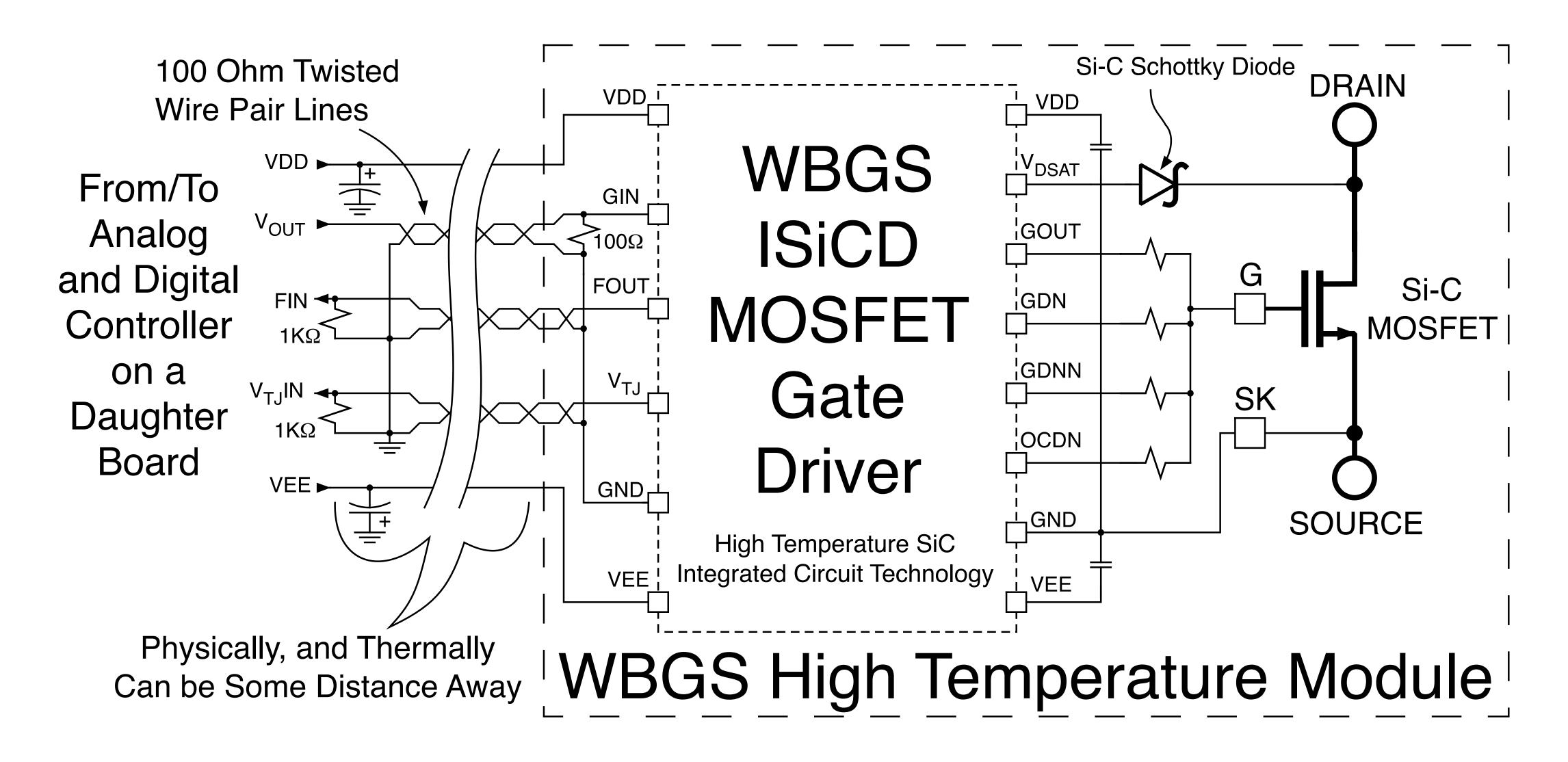
WBGS High Temperature ISiCD MOSFET Driver Co-Packaged With an SiC MOSFET
